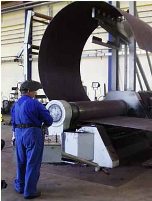
**Figure 11: Manufacturing Steel Tubular Sections**
