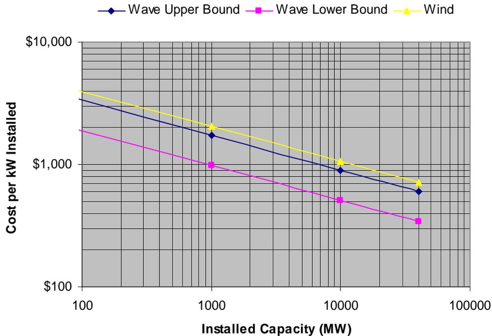
**Figure 30: Installed Cost per kW installed as a Function of Installed Capacity**
