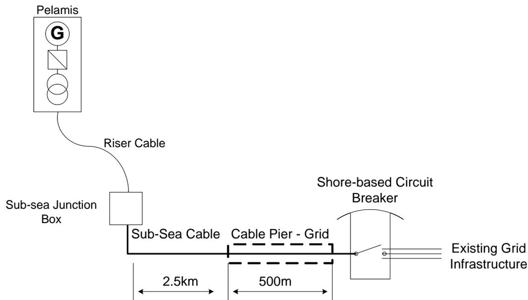
**Figure 18: Electrical Interconnection of a 1 Pelamis Pilot Plant**
