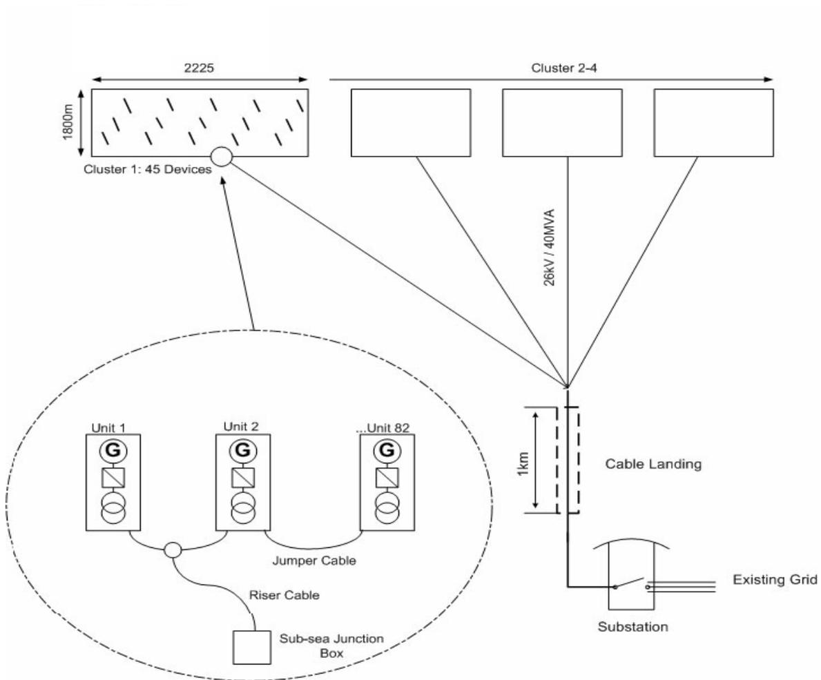
**Figure 19: Overall System Layout and Electrical Connections**
