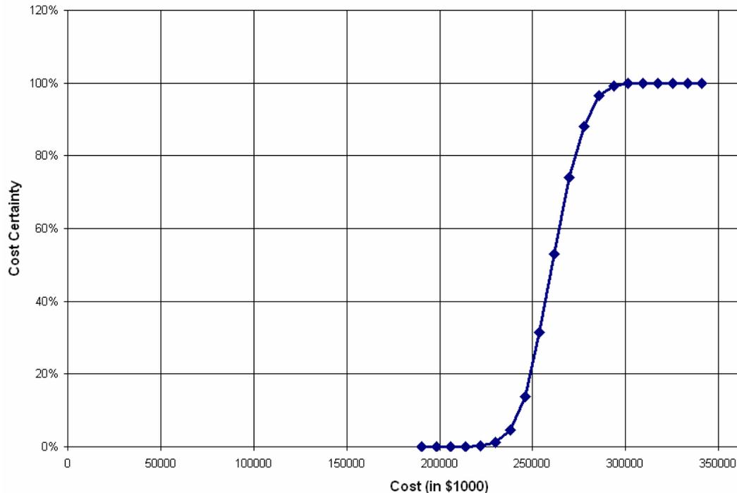
**Figure 24: Installed Cost uncertainty S-curve**
