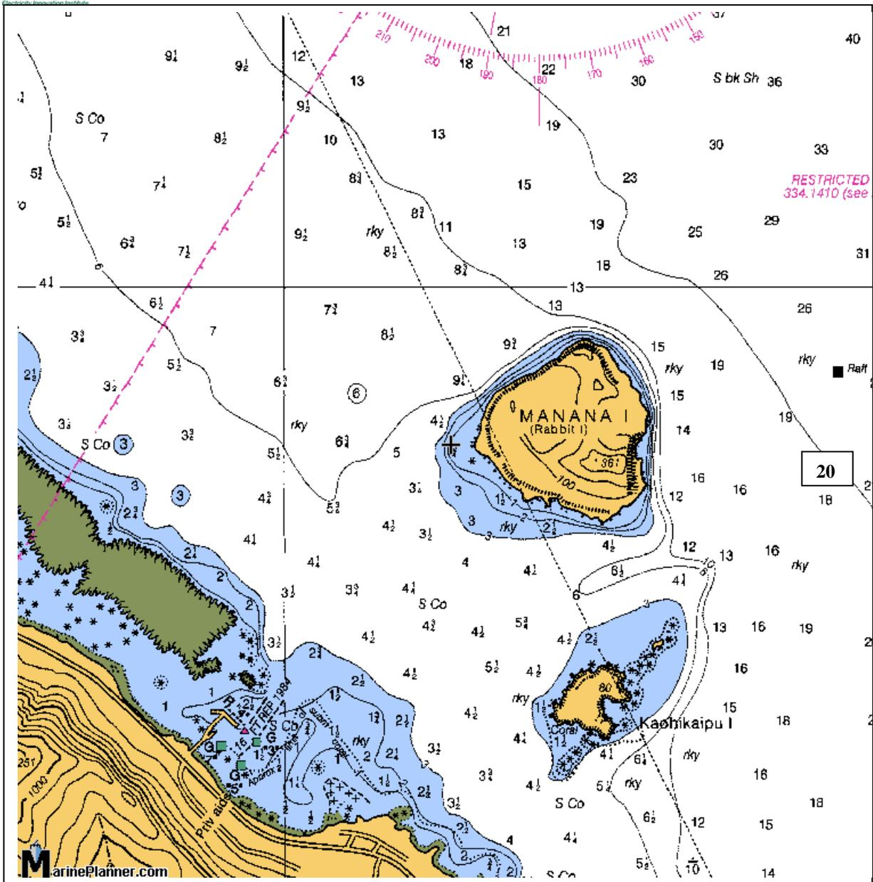
Figure 5: Local Bathymetry map showing the water depth in fathoms (1 fathom = 6 feet)
