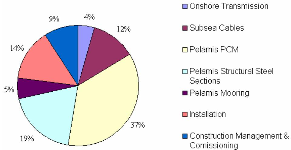
**Figure 21: Pie Chart of cost centers for single unit installation**
