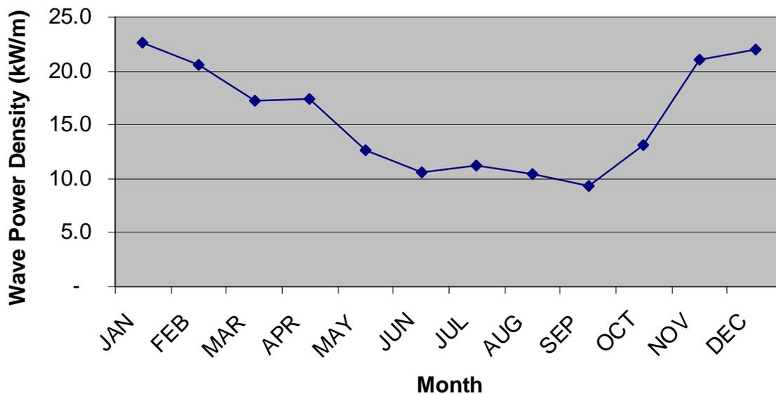
Figure 6: Monthly Average Wave Power Flux (kW/m)
