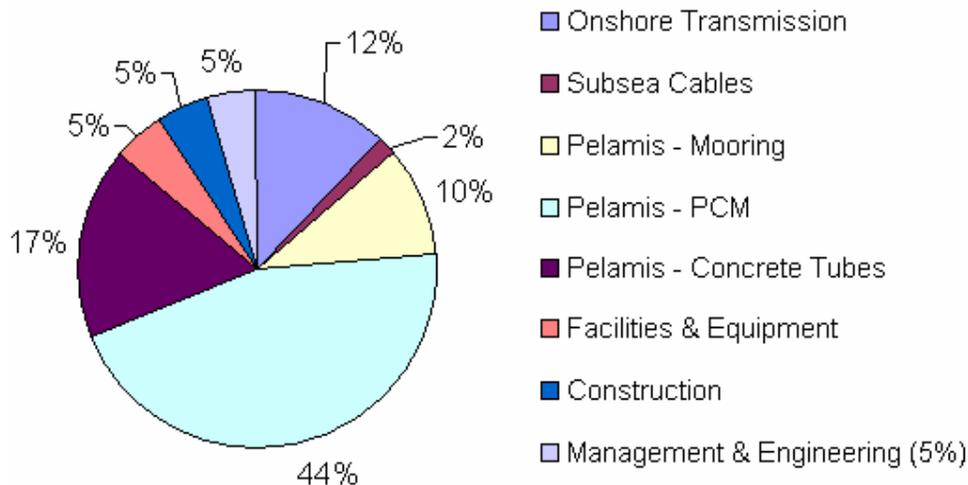
**Figure 23: Installed Cost Breakdown for commercial scale plant**
