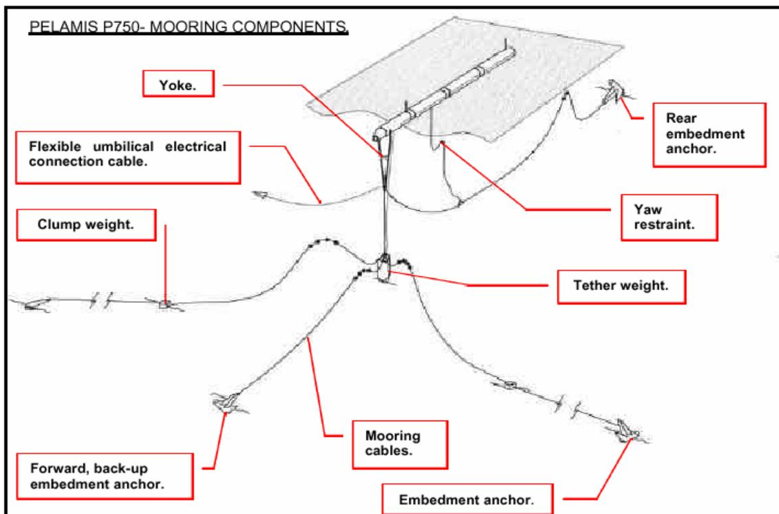
**Figure 12: Mooring Arrangement of Pelamis**
