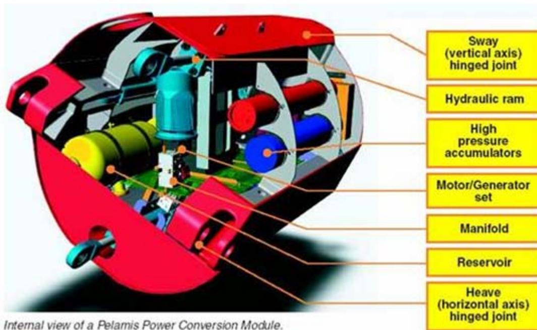
**Figure 10: Internal View of the Pelamis PCM**
