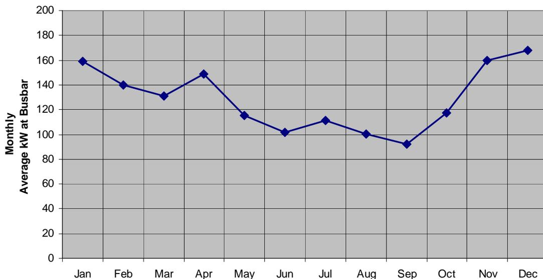
**Figure 20: Monthly average power delivered to bus bar – Pilot Plant**
