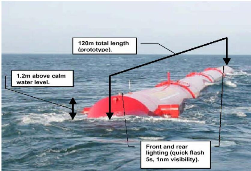
**Figure 7: Pelamis pre-production prototype undergoing sea-trials**
